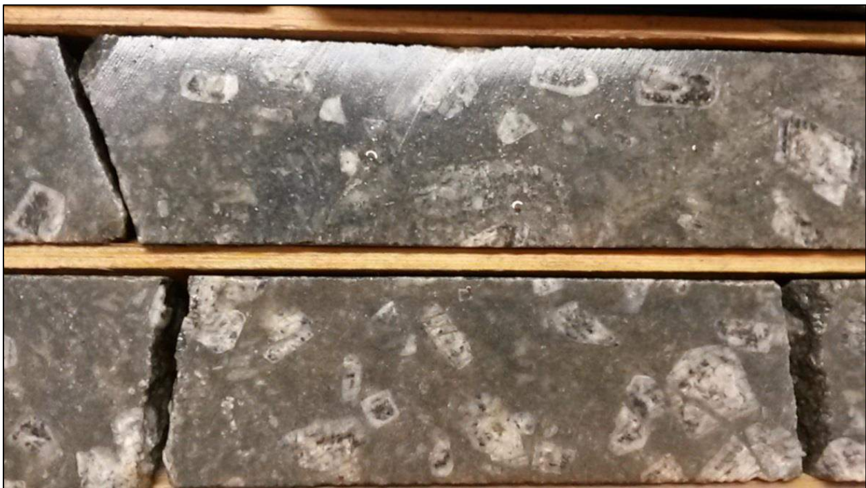
Figure 7-5 Porphyry with large Phenocrysts of Feldspars
