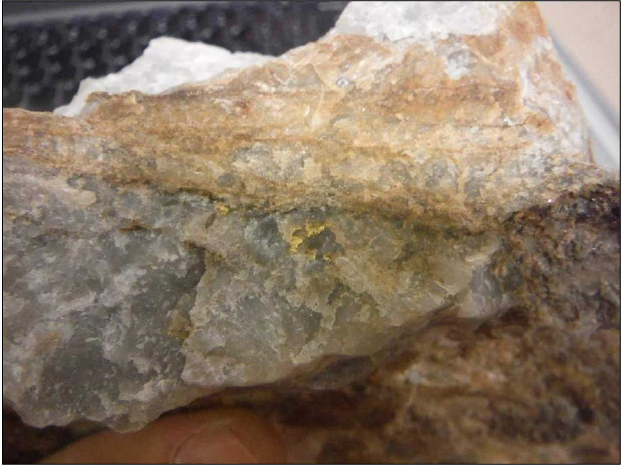
Figure 7-6 Visible Gold Within Smoky Quartz Vein in a Surface Sample
