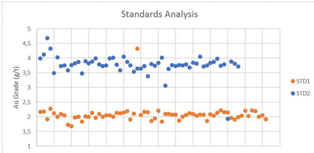
Figure 11-2 Distribution of standards (Au g/t) used in the 2016 drilling campaign
